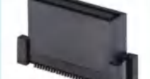
3725系列 0.8mm 浮动式BTB公头 Spec: 0.8mm floating Board to Board Connector Male Header SMT Height: 13.4mm Positions: 20-100P
