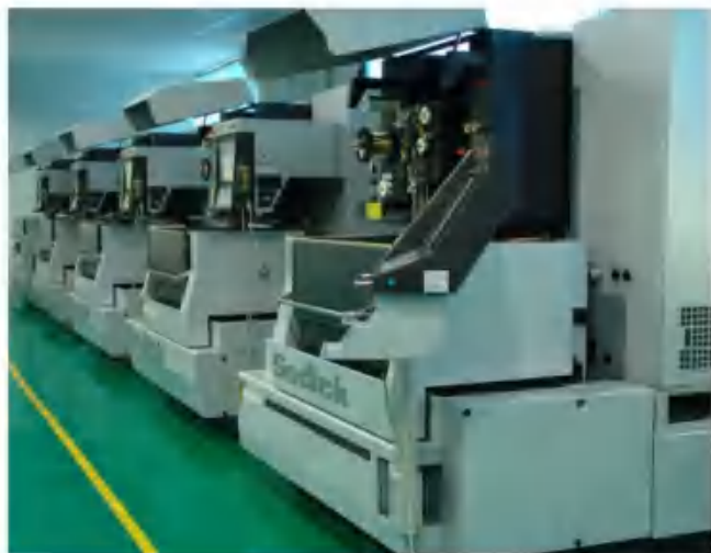
夏米尔，沙迪克精密 慢走丝线切割机 Sodick low-speed wire cutting machine Mould production
