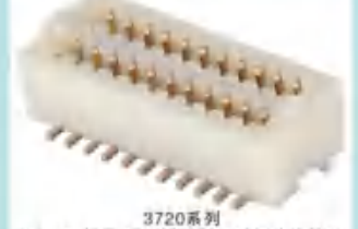
3720系列 0.5mm 间距 板对板双面接触母头连接器 Spec:0.5mm Pitch Board to Board Connector Double Contact Female Height:3.0/3.5/4.0/4.5/5.0/5.5/6.0/6.5mm Positions:10-100P
