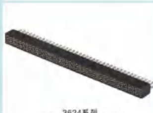
3624系列 1.27mm圆孔座 双排180度 Spec: 1.27mm Pitch Machined Female header Straight H3.8 mm Dual Row Positions: 2 × 2P-2 × 50P
