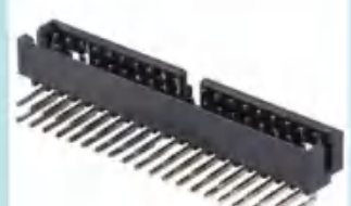
3221系列 2.0mm 筒牛90度 Spec:2.0mm Pitch Box header Right Angle H6.35mm Positions:6-64P
