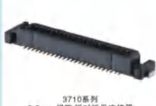
3710系列 0.8mm 间距 板对板公头连接器 Spec:0.8mm Pitch Board to Board Connector Male Height:4.8mm Positions:40P
