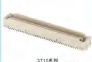
3710系列 0.8mm 间距 板对板公头连接器 Spec:0.8mm Pitch Board to Board Connector Male Height:4.6/7.6mm Positions:40-120P
