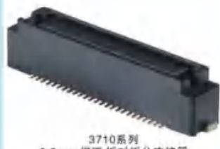
3710系列 0.8mm 间距 板对板母头连接器 Spec:0.8mm Pitch Board to Board Connector Female Height:5.1mm Positions:40P
