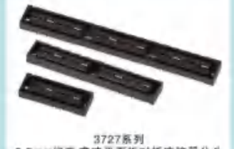
3727系列 0.5mm 间距 高速平面板对板连接器公头 Spec:0.5mm Pitch High-speed Board to Board Male Connector Height: 3.25mm Positions: 60P
