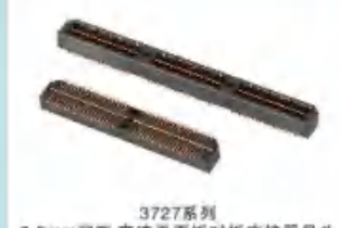
3727系列 0.5mm 间距 高速平面板对板连接器母头 Spec:0.5mm Pitch High-speed Board to Board Female Connector Height: 4.06mm Positions: 60P
