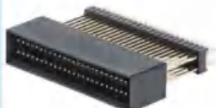
3242系列 1.27x2.54mm 筒牛180度+排针胶芯 Spec:1.27x2.54mm Pitch Box header Straight Add Pin Headr Plastic H10.0mm Positions:10-100P
