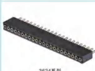
3624系列 1.27mm圆孔座 单排180度 Spec: 1.27mm Pitch Machined Female header Straight H4.1 mm Positions: 1 × 2P-1 × 50P
