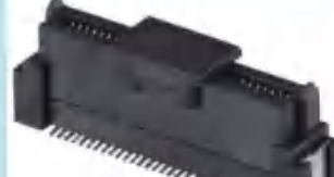
3711系列 0.8mm 间距 板对板D型母头连接器 Spec: 0.8mm Pitch Board to Board D-type Female Connector Height: 7.4/10.4/11.4/12.4/13.4mm Positions: 20-120P
