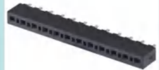
2989系列 3.96mm 排母单排180度 Spec:3.96mm Pitch Female header Single Row Straight H8.9mm Positions:1×2-1×20P
