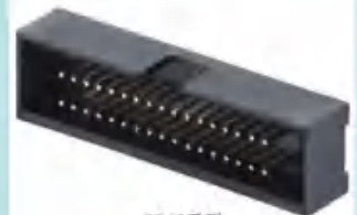
3240系列 1.27x2.54mm 筒牛中间带缺口180度 Spec:1.27x2.54mm Pitch Box header With Middle Notch Straight H5.6mm Positions:10-100P
