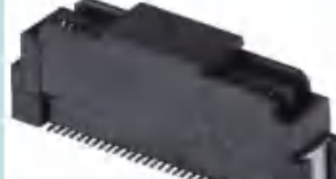
3711系列 0.8mm 间距 板对板D型公头连接器 Spec: 0.8mm Pitch Board to Board D-type Male Connector Height: 8.0/11.0/12.0/13.0/14.0mm Positions: 20-120P
