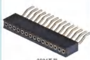
3624系列 1.27mm圆孔座 单排卧贴 Spec: 1.27mm Pitch Machined Female header Right Angle SMT H4.1 mm Positions: 1 × 2P-1 × 50P
