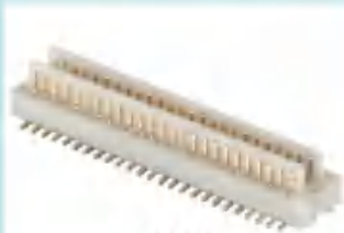
3713系列 0.8mm 间距 板对板双面接触公头连接器 Spec:0.8mm Pitch Board to Board Connector Double Contact Male Height:1.0/2.0mm Positions:8-100P
