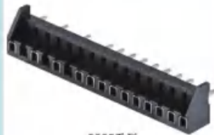
8525系列 2.54mm D型蜈蚣脚排母单排 Spec:2.54mm Pitch Female header Single Row D type bottom entry H5.0mm Positions:3-25P
