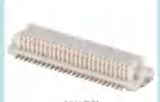
3720系列 0.5mm 间距 板对板公头带定位片连接器 Spec:0.5mm Pitch Board to Board Connector Male With Locating Plate Height:2.2mm Positions:10-80P
