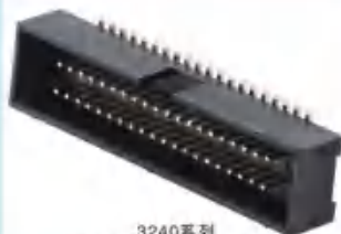
3240系列 1.27x2.54mm 筒牛SMT Spec:1.27x2.54mm Pitch Box header SMT H5.6mm Positions:10-100P
